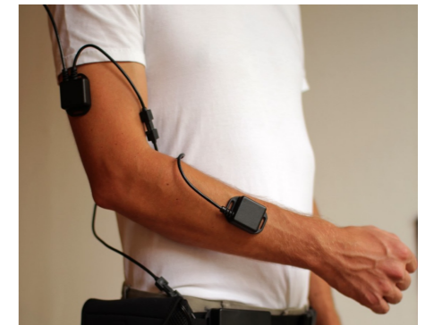
inertial: wearable IMU, MotionNode
