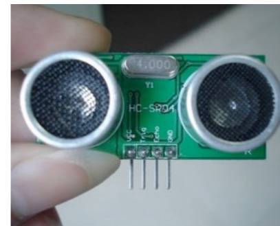
acoustic: ultrasonic proximity sensor, BiF
